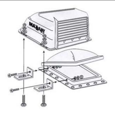
NOTE: All hardware provided with MaxxAir's Zero-Leak Mounting System is made of stainless steel or aluminum for durability and long life.Place the MaxxAir Vent Cover over the roof vent with the louver area facing the rear of the vehicle. After verifying that the Vent Cover is centered over the roof vent, trace on your roof (with a pencil) the location of the slots in the MaxxAir Vent Cover's mounting flange.
